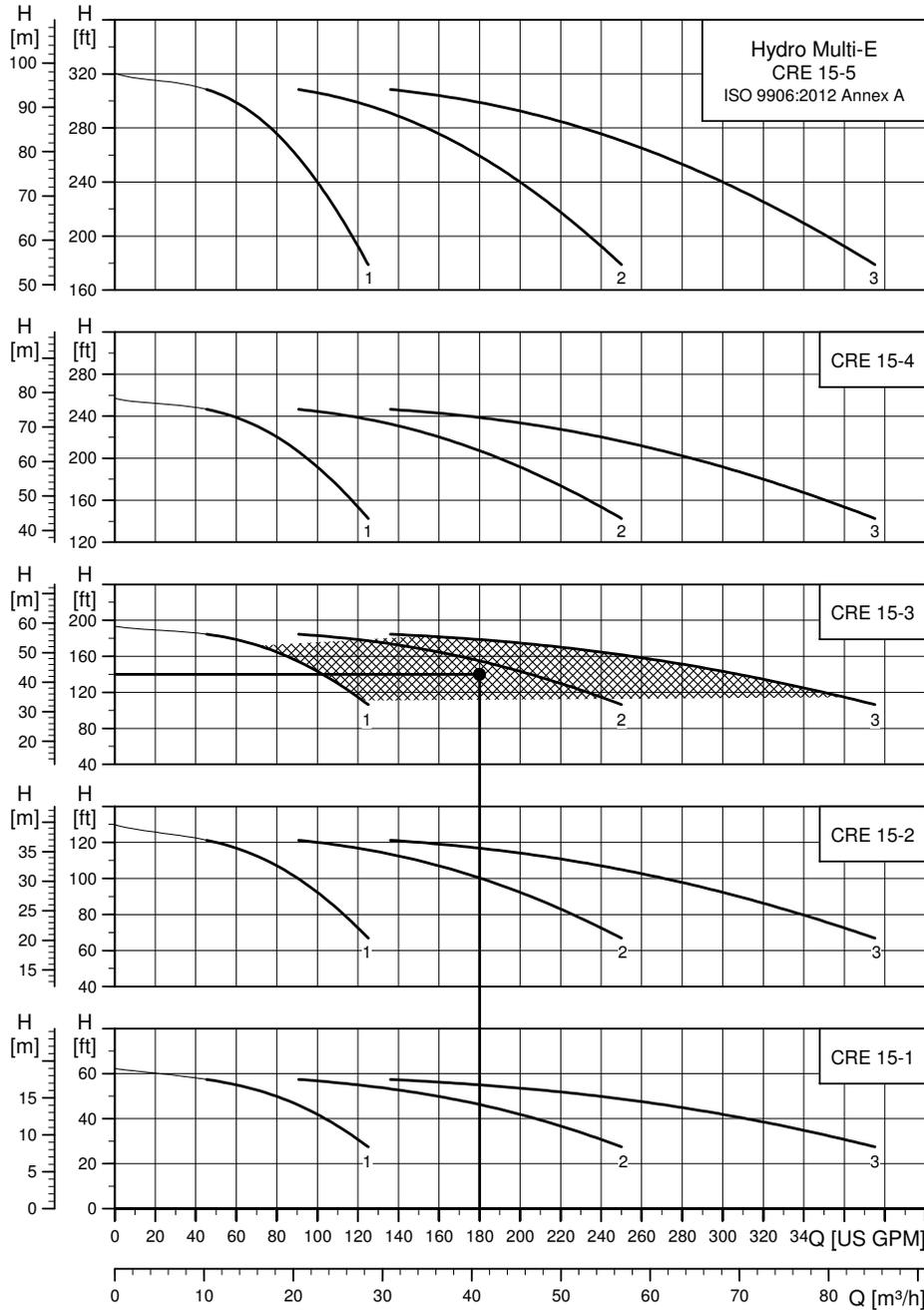
Fig. 20 Example of how to select a system
