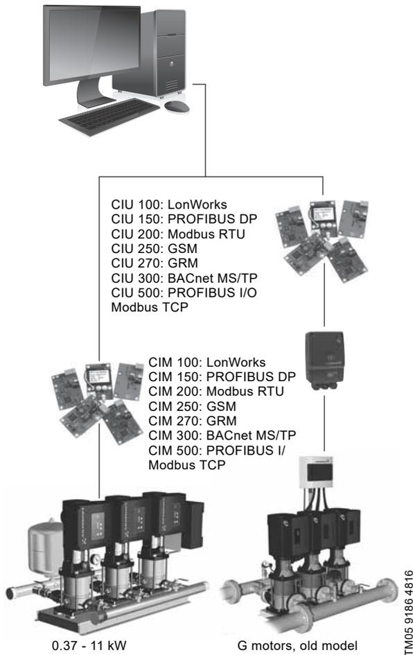
Fig. 13 Structure of a building management system
