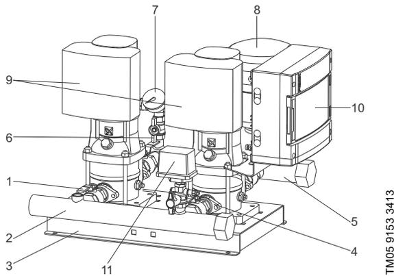
Fig. 4 Hydro Multi-E with two CRE pumps
